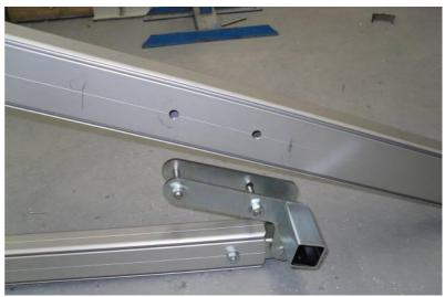
The roof rail is connected to corner post and secured using the 17mm spanners, This assembly is carried out with the parts still on the floor, repeat for each post.
