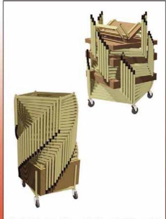
Standard storage dollies and trolleys should be used if purchased. Position the decks to the bottom of the spiral in order to keep the centre of gravity low (see above left). If this causes access problems, keep a few decks you might need towards the top, or stack decks then frames in small numbers alternately (see above right).
