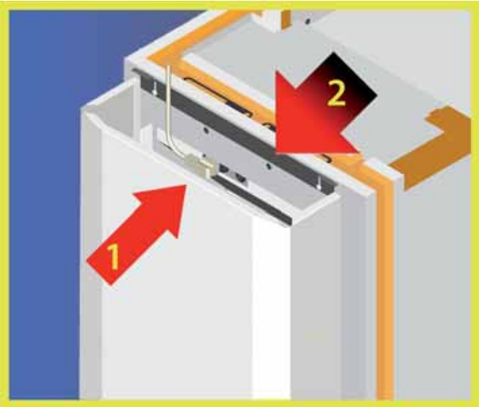
Pic. 15. Installation of the cable and upper front cover.
