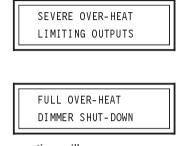
Normal operation will resume as soon as the internal temperature of the dimmer has reduced.
