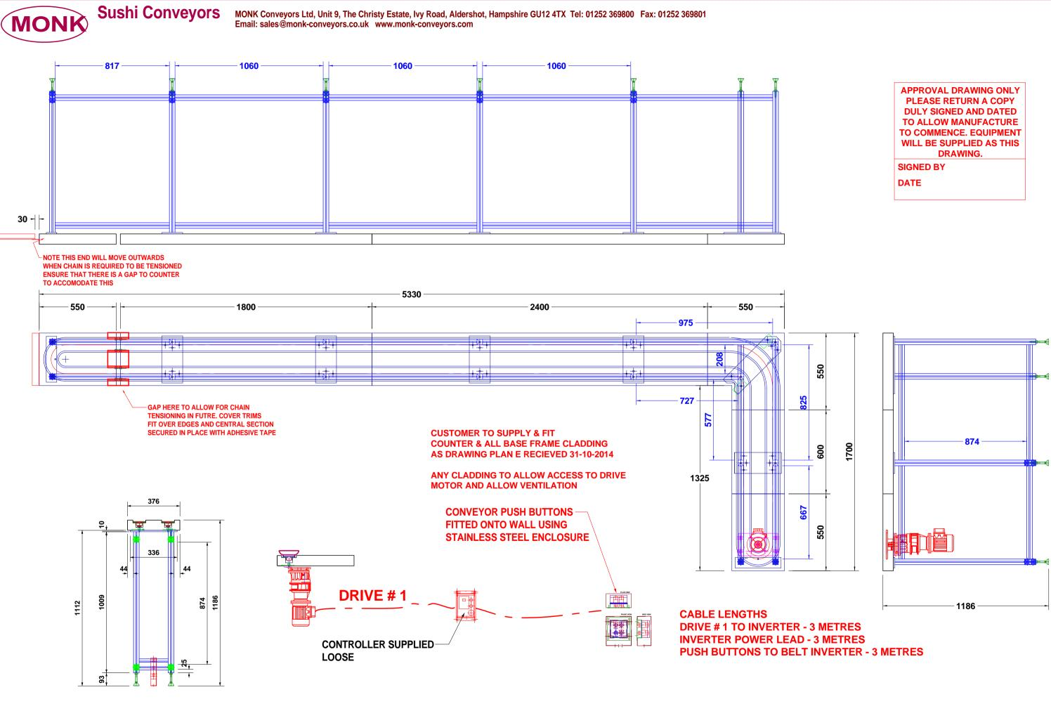
Iss 2 (7/11/2014 JS) O/ALL LENGTH INCREASED BY 30mm TO ALLOW FOR CHAIN TENSIONING
